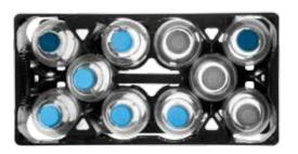
They cause obstructions in the unpacker if they are out of shape, defective, dirty or the incorrect brand. The efficiency and productivity of complete filling lines are also affected if they contain too many non-brand bottles: therefore it is necessary that returned returnable bottle crates with such faults are detected and sorted out in good time – with the HEUFT *LGX*! It examines their dimensions and complete insides optically
