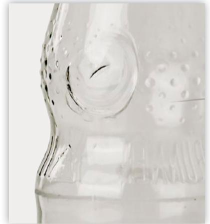
The HEUFT InLine IX identifies glass splinters, thread cracks and shell-shaped fractures, to name but a few.
