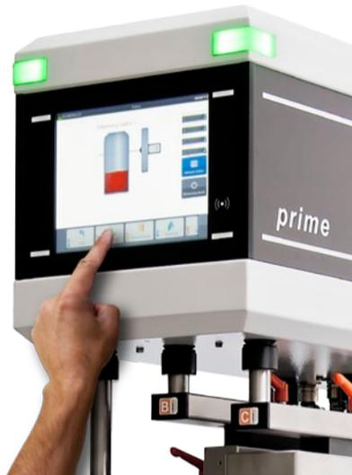
Inspecting the fill level and measuring the internal pressure, checking the presence, position and tightness of closures, detecting unlabelled containers, burst bottles and serial faults, consistently rejecting faulty drinks packaging: the HEUFT *prime* with its modular design provides all the functions which a full container check requires.
