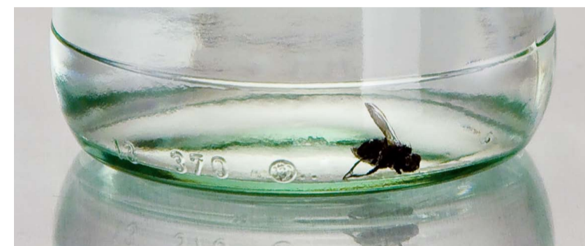
A perfected inspection procedure minimises the risk of low density foreign objects, such as this insect on the bottom of the bottle, being overlooked.
