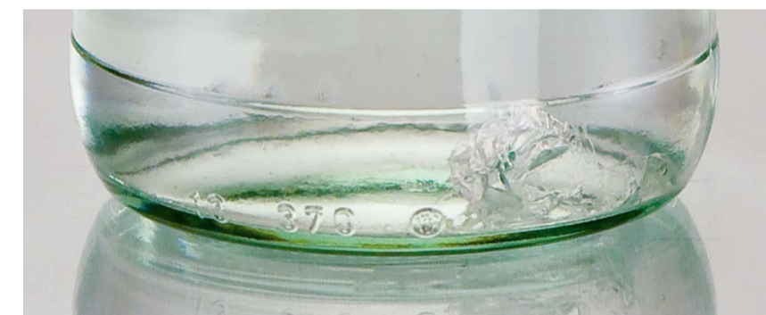
Transparent foil is one of the faults which can now be detected even on parts of the base which are difficult to inspect.
