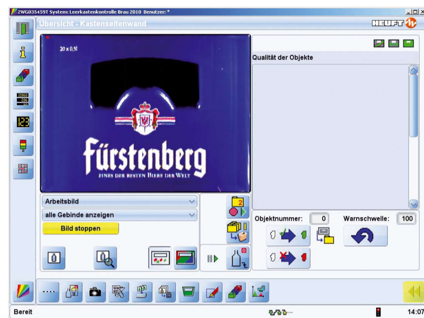
A general view is displayed on the HEUFT PILOT graphical user interface at the operating terminal of the HEUFT LGX. It shows the complete sidewall of the empty crate without wasting the picture area.
