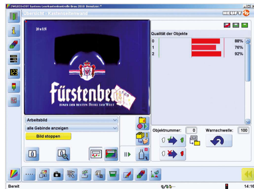
Label remains and other objects which deviate from the standard can be perfectly identified in the high-resolution photograph. The system marks them independently and submits an initial assessment whether and with what probability these are real faults. The final decision then lies with the operator.
