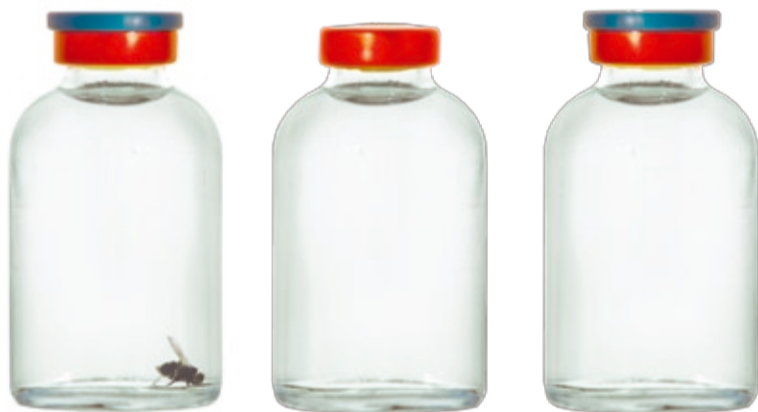
Foreign objects as well as the incomplete or faulty elements of crimp caps and other types of closures are clearly identified.
