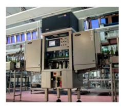
The additionally integrable sidewall inspection carries out a continuous inspection of the empty bottles.
