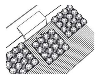
The **HEUFT** *maxi-flip* rejects empty, half-full or completely full cases each an equal distance onto parallel conveyor chains. Its rejection segment is activated for a longer time for heavy cases or cardboard boxes than for lighter ones. A complex mechanical changeover for different types of cases is not necessary.
