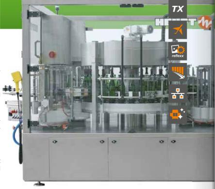
HEUFT TORNADO flex servo technology for a fine adjustment of each individual bottle with millimetre accuracy.
