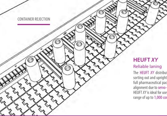
The HEUFT XY distributes containers onto up to four lanes. The sorting out and upright rejection of different shapes of empty and full pharmaceutical packaging is achieved without changing their alignment due to servo-controlled rejection segments. Therefore the HEUFT XY is ideal for use on pharmaceutical lines with a performance range of up to 1,000 containers per minute.
